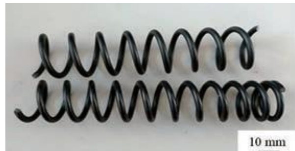
Fig1. Spring compressed and partially broken after electrophoresis
